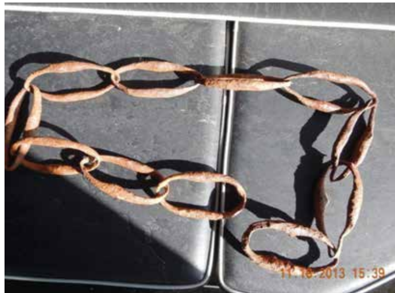
Picture 4: Example of a worn mooring chain
